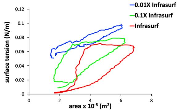
**Supplemental Figure 11. Constrained drop surfactometer used to measure surfactant function.** A) Constrained drop surfactometer (CDS) fabrication schematic. Droplet stage (a) is threaded into pedestal (b), with interior channels (c) continuous with syringe pump tubing port (d). B) CDS is placed upon goniometer stage for droplet recording. C) Surface tension vs surface area plots of serial dilutions of Infracurf measured by surfactometry.
