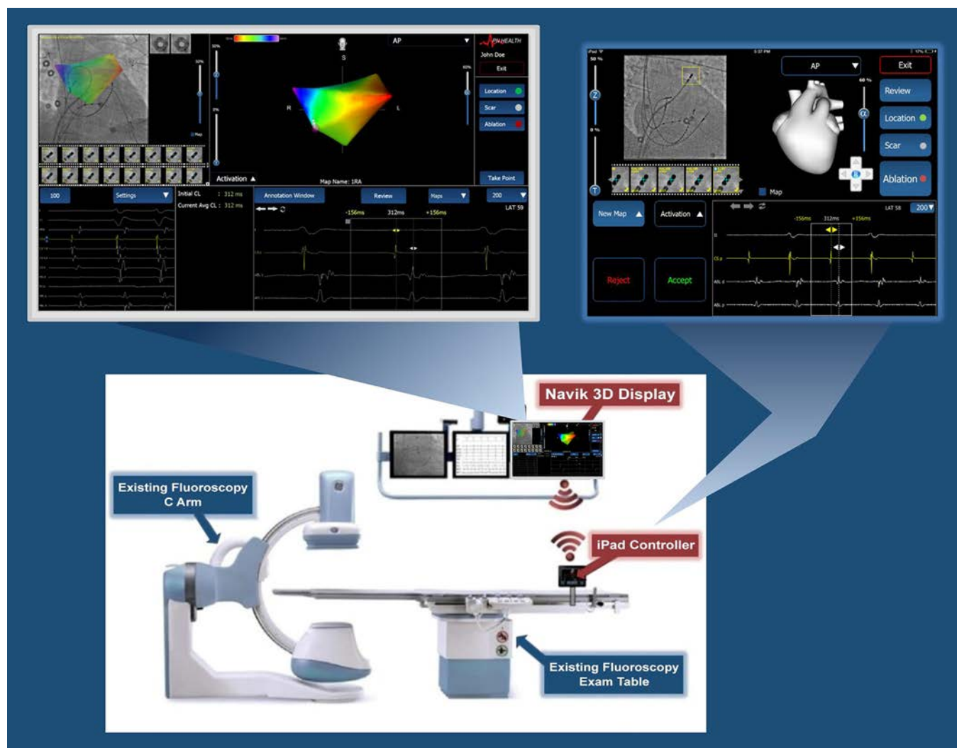
Figure 1. Navik 3D in the context of the electrophysiology lab. Navik 3D utilizes data from existing fluoroscopy and electrocardiogram-electrogram equipment to generate 3D cardiac maps for use during electrophysiology procedures. The system provides 2 user interfaces (U/I) to the interventional team: (i) Main application U/I (upper left) generated by the system's Main computer workstation, which displays real-time fluoroscopy images and the 3D cardiac map, and (ii) a U/I on the Apple iPad (upper right), which serves as controller only and enables physician-directed operation from any location in the electrophysiology lab. AP, anteroposterior; CL, cycle length; LAT, local activation time.
